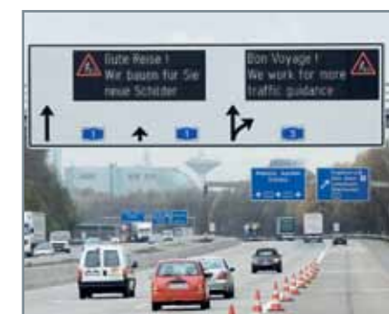
Combination of limited / freely programmable variable message sign, multicolor graphical display / monochrome text lines
