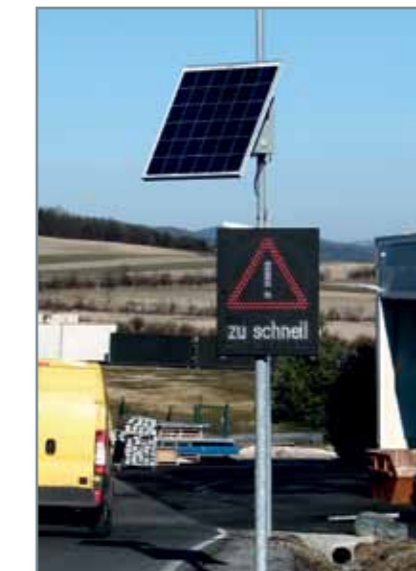
Radar activated/limited variable message sign powered by PV panel, bicolor Austria
