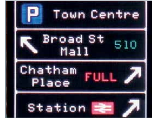
Freely programmable parking guidance display, UTMC communication protocol, full matrix, full color RGB, 16 mm pixel pitch United Kingdom
