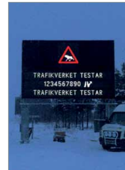
Freely programmable, RGB graphical area (top); white, fully graphical text lines (bottom), Sweden
