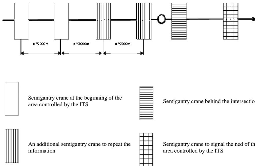
**Fig. 2.** Example of installation of variable message signs on the section of road covered by a traffic management system
