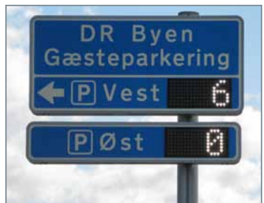
3-character display, white LED, 160 mm character height, 3 LEDs in 1 pixel
