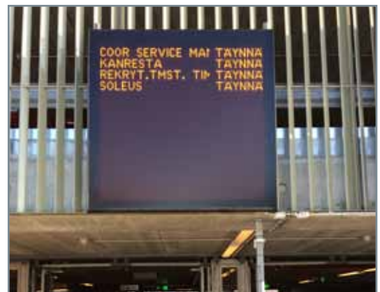
Fully graphic display, total resolution 160 x 168 pixels, pixel pitch 8 mm, monochrome
