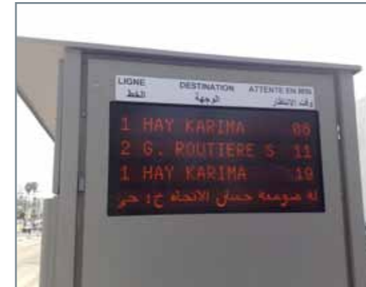
4-line display, single sided, resolution 192x16 pixels/line, pixel pitch 4 mm, communication Ethernet
