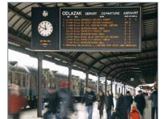
10-line display, single sided, resolution 288x8 pixels/line, pixel pitch 8 mm, communication Ethernet, analog clock
