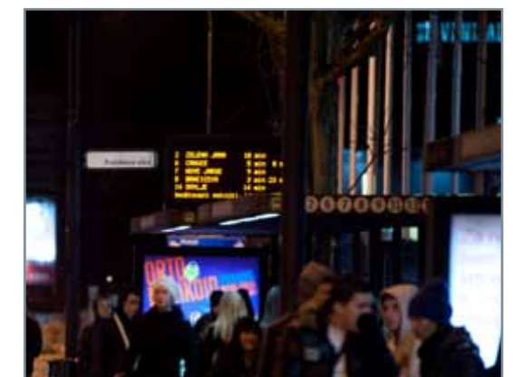
2- and 6-line display, single sided, resolution 192x8 pixels/line, pixel pitch 4 and 6 mm, communication Ethernet/GPRS/Zigbee
