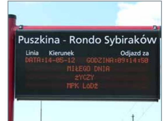
4-line display, double sided, resolution 192x8 pixels/line, pixel pitch 6 mm, communication Ethernet, pre-recorded audio, silk print
