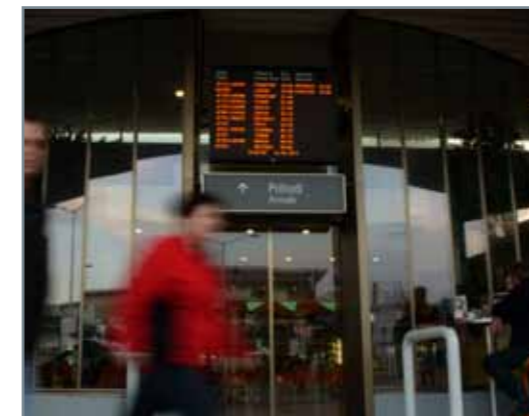
13-line display, single sided, resolution 288x8 pixels/line, pixel pitch 4mm, communication Ethernet
